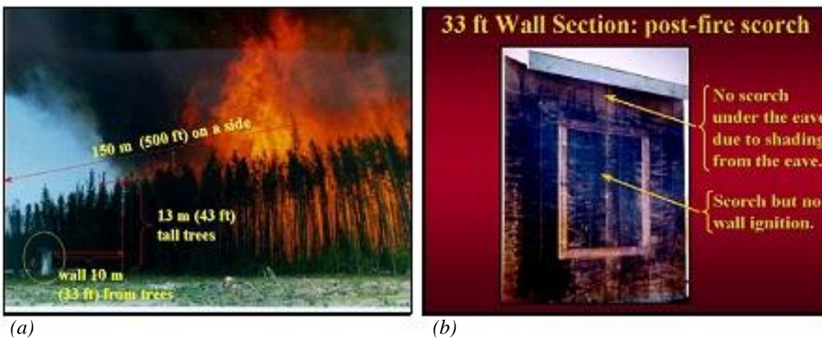
Figure 2—Home ignition research over the last several years has exposed wall sections to crown fires. (a) Wall sections were placed at 33, 66, and 98 feet from the forest edge. (b) Ignition of the 33 ft wall section occurred during 3 out of 7 crown fires. No ignitions or significant scorch occurred on wall sections at 66 ft and 98 ft during any crown fire.
