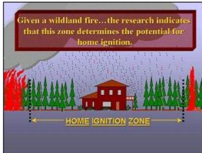
Figure 3—The home ignition zone includes the home and an area surrounding the home within 100 to 200 feet. The potential for ignition depends on the home's exterior materials and design and the amount of heat to the home from the flames within the home ignition zone. Firebrand ignitions also depend on the home ignition zone either by igniting the home directly or igniting adjacent materials that heat the home to ignition.
